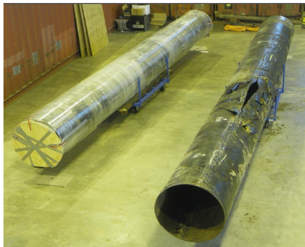
Picture 1 – This picture shows one of the rusted and punctured pipelines from the Southern Oil and Gas fields in Angola and a modern hard coated geothermal pipeline from Enbridge Inc.to replace it
