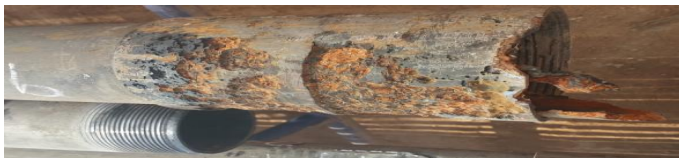
Fig.4: Uniform General and localized Corrosion due to CO 2 resulting in Metal wastage and pitting
