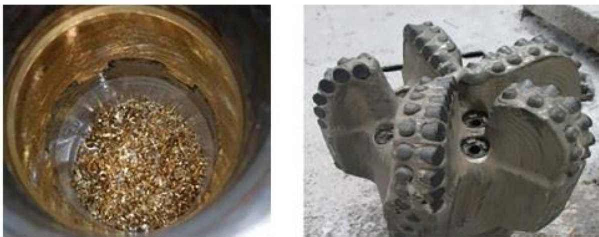
Figure 2 – XCD bit drilled in laboratory tests (left), SDi516 bits, no wear after XCD drilling in a field in Western Siberia.
