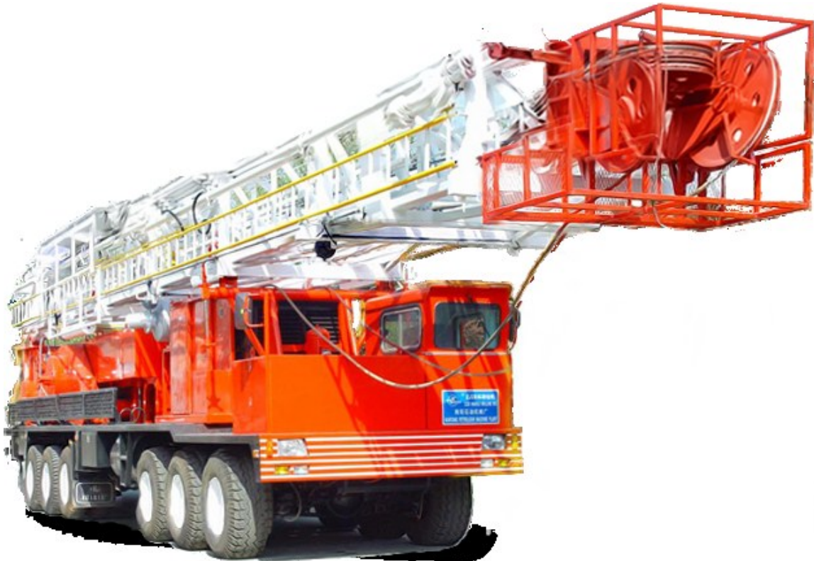
Figure 3. Mobile drilling installation XJ1000
